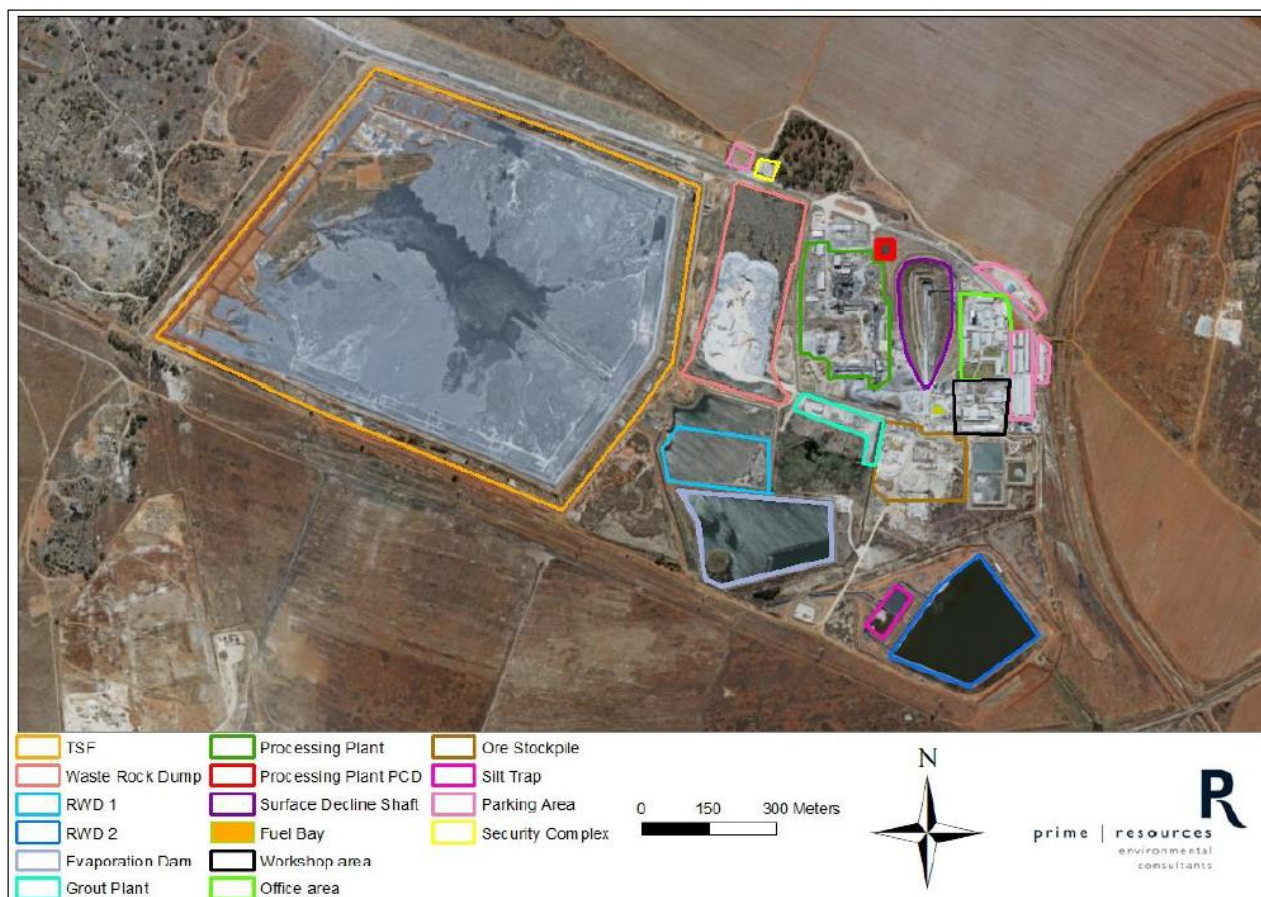
Figure 1: Layout of the New Kleinfontein Gold mine (2022 IWWMP).
